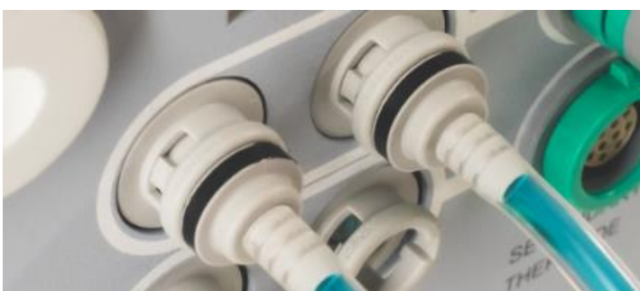
Figure 20: Wrong coolant connectors' connection should be rotated all the way clockwise
