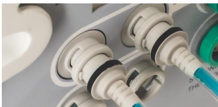
Figure 19: Wrong coolant connectors' connection should be inserted all the way in
