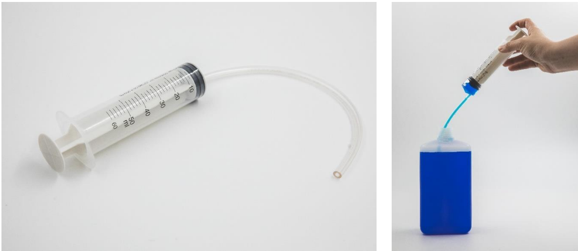
Figure 16: Filling the syringe with coolant liquid
