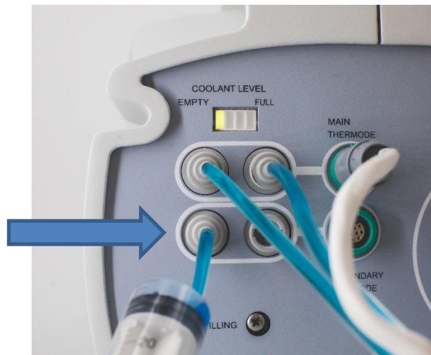
Figure 18: Connecting the syringe to the system
